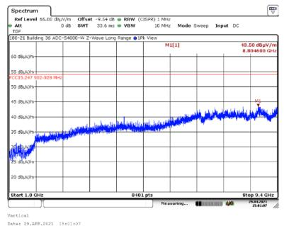
A4.6.2. Measurement Results: Vertical Antenna
