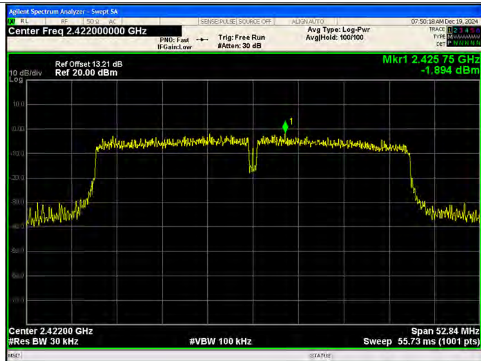
PSD NVNT n40 2422MHz Ant1
