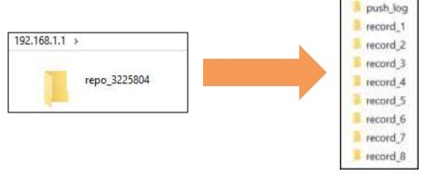
(5) Double click the folder that you have configured to store the static data, you will see the folder(s) created by the eBase system automatically and named by the date which is decide by GPS time when you start to log data.
