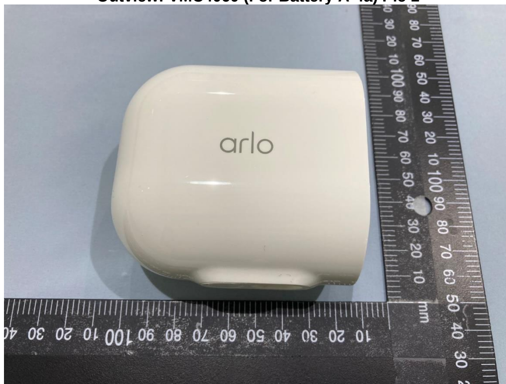
Outview: VMC4060 (For Battery A-4a) Pic 1
