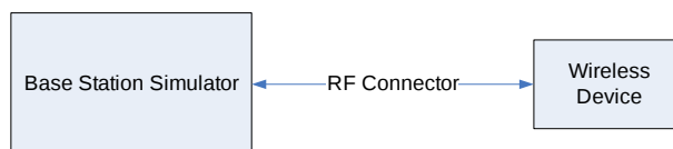
Figure 9-1 Power Measurement Setup
