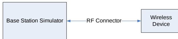
Figure 9-3 Power Measurement Setup
