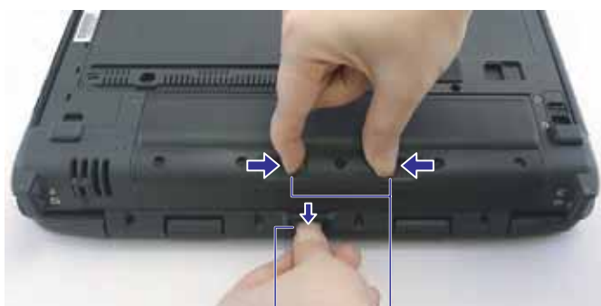
Press down Battery Lock Battery Release Latches
