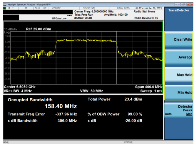
Plot 7-128. 26dB & 99% Bandwidth Plot Antenna 1b (160MHz 802.11ax RU996x2 (UNII Band 6) – Ch. 111)
