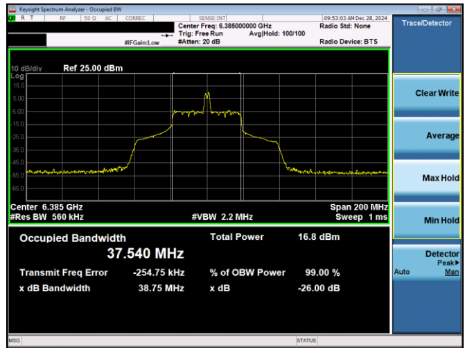
Plot 7-115. 26dB & 99% Bandwidth Plot Antenna 1b (80MHz 802.11ax RU26 (UNII Band 5) – Ch. 87)
