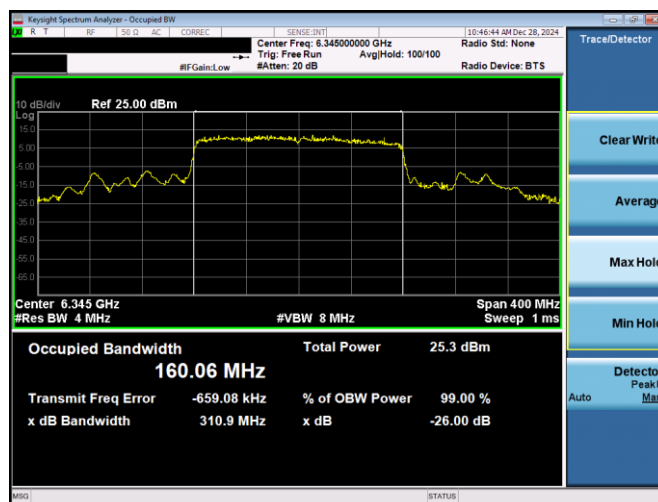
Plot 7-120. 26dB & 99% Bandwidth Plot Antenna 1b (160MHz 802.11ax RU996x2 (UNII Band 5) – Ch. 79)
