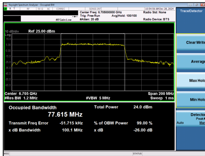
Plot 7-135. 26dB & 99% Bandwidth Plot Antenna 1b (80MHz 802.11ax RU996 (UNII Band 7) – Ch. 135)
