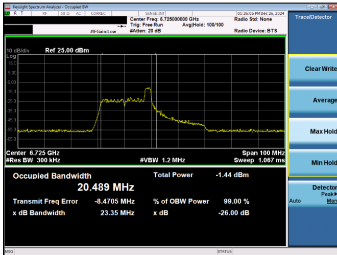
Plot 7-154. 26dB & 99% Bandwidth Plot Antenna 1b (40MHz 802.11ax RU26 (UNII Band 7) – Ch. 155)
