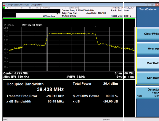
Plot 7-134. 26dB & 99% Bandwidth Plot Antenna 1b (40MHz 802.11ax RU484 (UNII Band 7) – Ch. 155)
