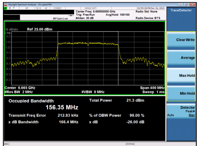
Plot 7-160. 26dB & 99% Bandwidth Plot Antenna 1b (160MHz 802.11ax RU996x2 (UNII Band 7) – Ch. 143)
