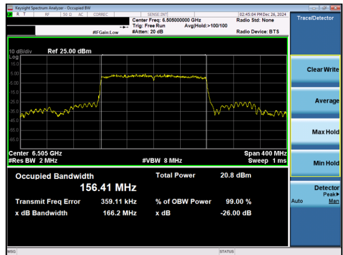
Plot 7-152. 26dB & 99% Bandwidth Plot Antenna 1b (160MHz 802.11ax RU996x2 (UNII Band 6) – Ch. 111)
