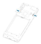
3. Insert the battery, making sure the connectors align.
