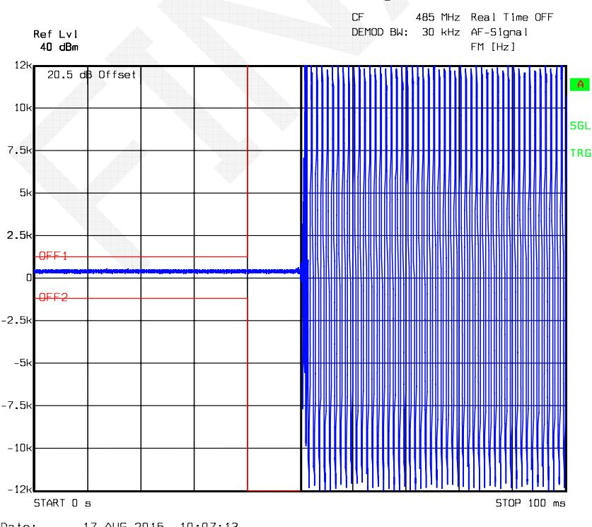
**Turn on – 485 MHz, 4FSK, High power level**
