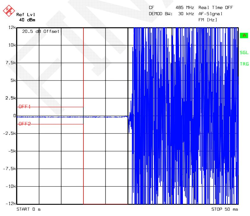
**Turn on – 485 MHz, 4FSK, Low power level**
