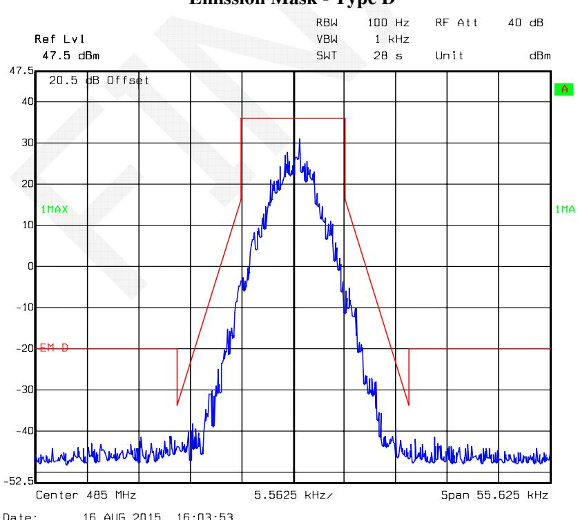
**Occupied Bandwidth – 4FSK, 485 MHz, Low Power Level**
