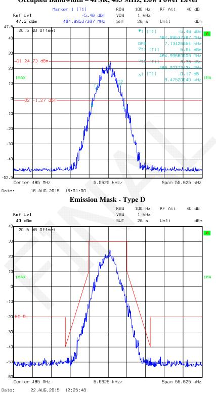
Occupied Bandwidth - 4FSK, 485 MHz, Low Power Level
