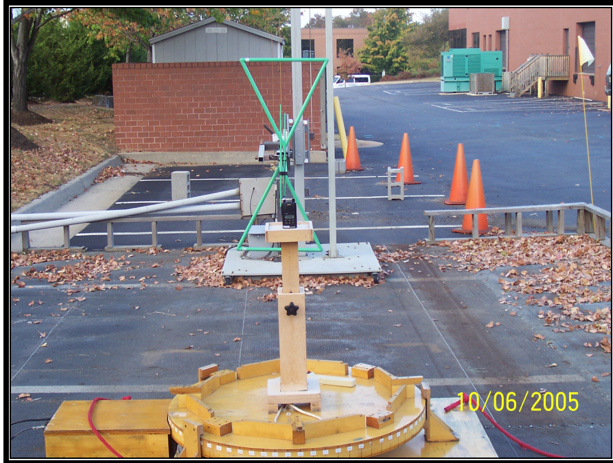
Photograph 3: Radiated Emissions Test Configuration (Front View)
