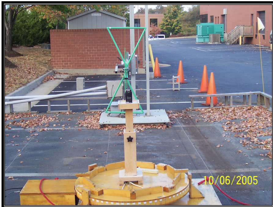
Photograph 4: Radiated Emissions Test Configuration (Rear View)
