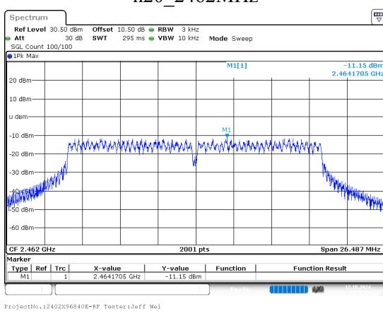
**5.7 100 kHz Bandwidth of Frequency Band Edge****Test Information:**
