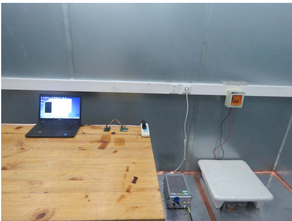
Picture 2 Conducted Emission Test Setup
