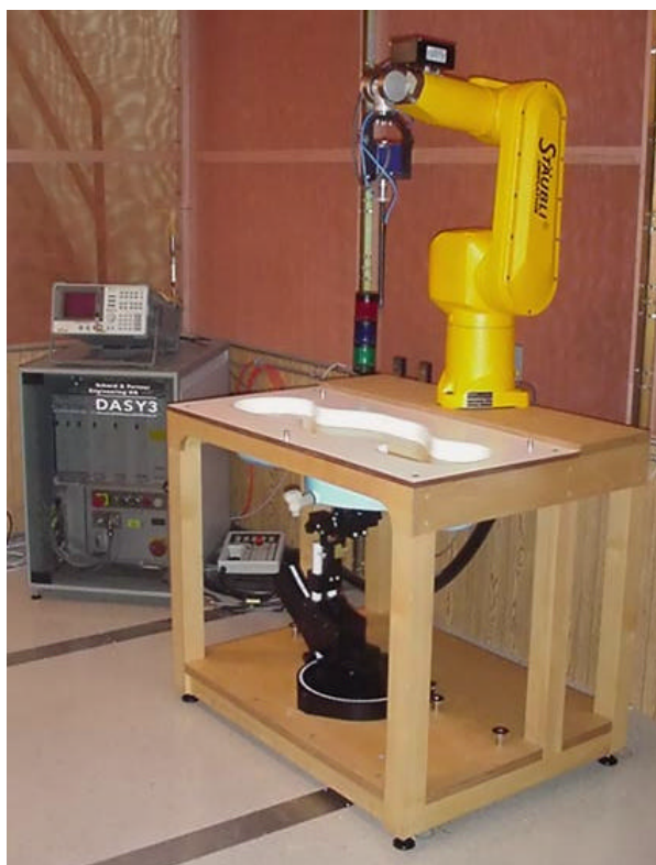
Fig. 5. DASY3 SAR Measurement System
