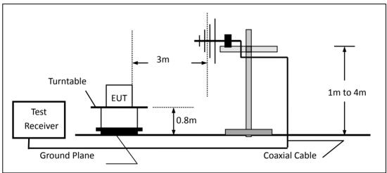
(c) For radiated emissions above 1000MHz
