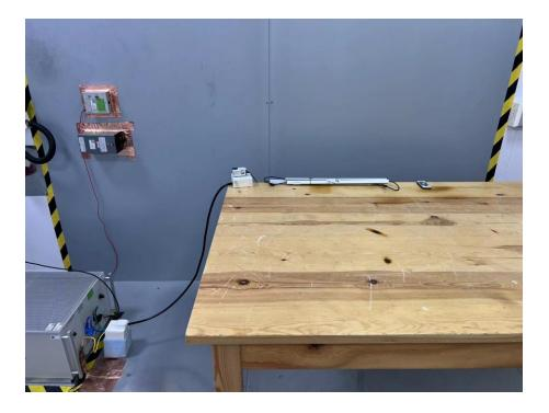
Set-up for Radiated Emission (RE), Below 1GHz
