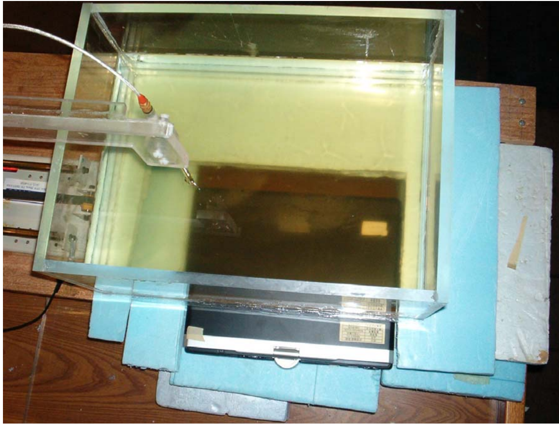
Fig. 6. Photograph of the Toshiba PC with top cover open and the back side of the top cover placed parallel to the bottom of the phantom at a distance of 2.5 cm. This is Configuration 3 for SAR testing and represents the case of a bystander at a distance of 2.5 cm from the back of the cover of the Toshiba Model PP350X-XXXXX Wireless PC.
