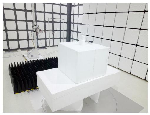
Description: Radiated Emission Test Setup for 18GHz~40GHz
