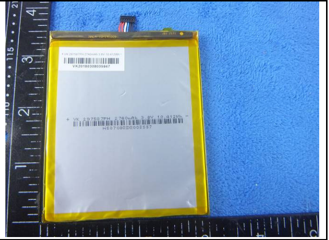
Battery - Front View
