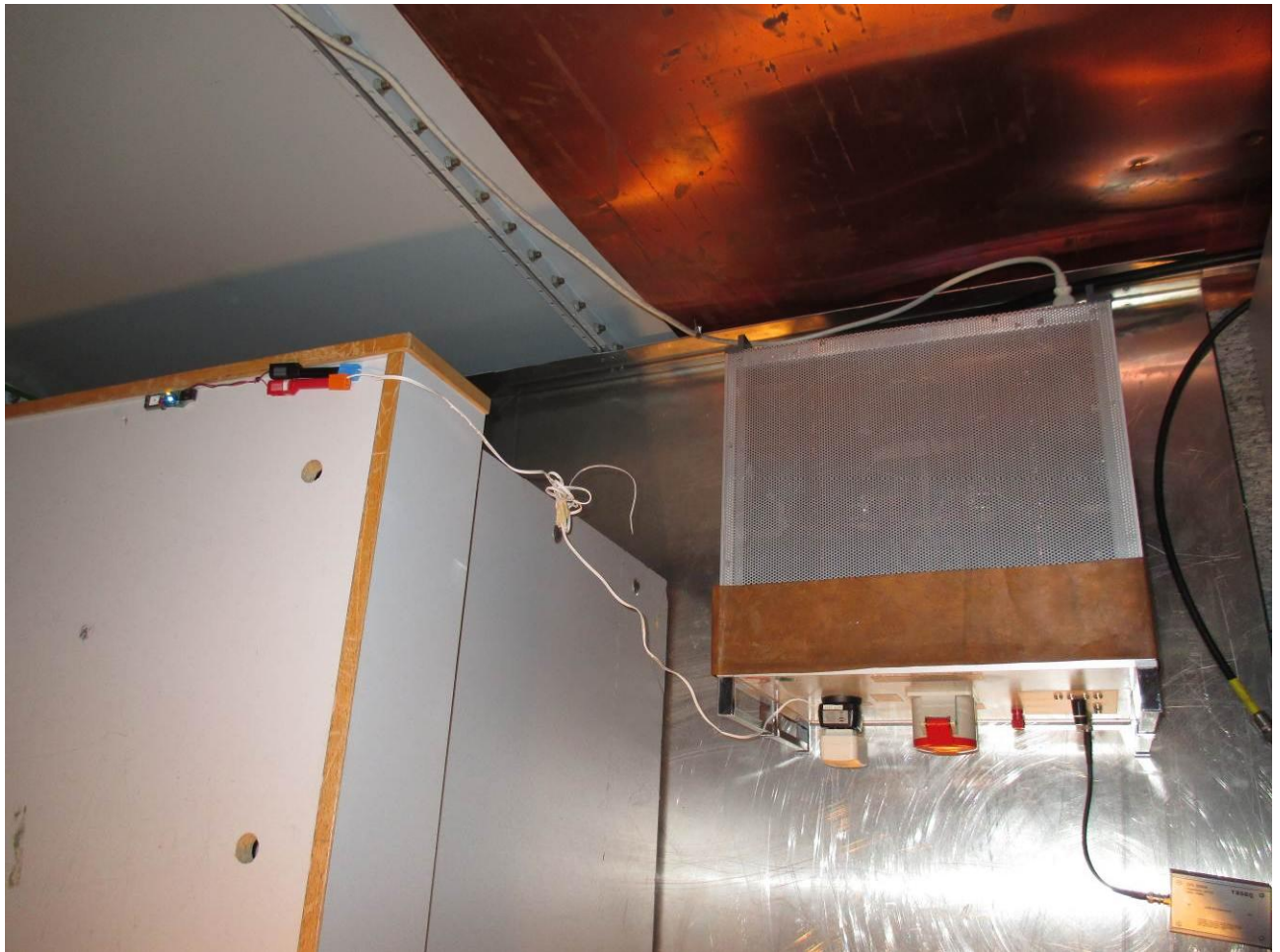
151496_20: Test setup – conducted emissions on power supply lines
