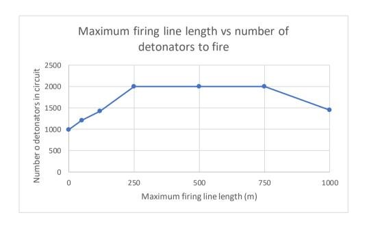
Each group of 200 DT5 detonators is spread over 1 000 m of bus line (detonator lead wire length of 15 m with HD2 wire type)
