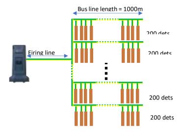
This is a typical connection diagram use case which could vary according to customer's deployment practices and operational setups.
