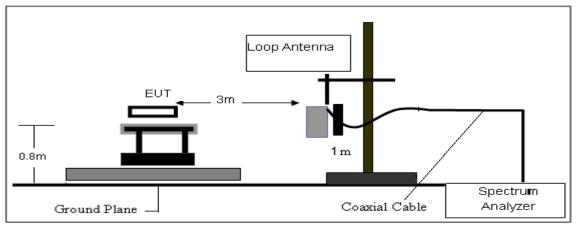
(B) Radiated Emission Test-Up Frequency 30MHz~1GHz
