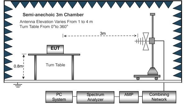
(C) Radiated Emission Test-Up Frequency Above 1GHz
