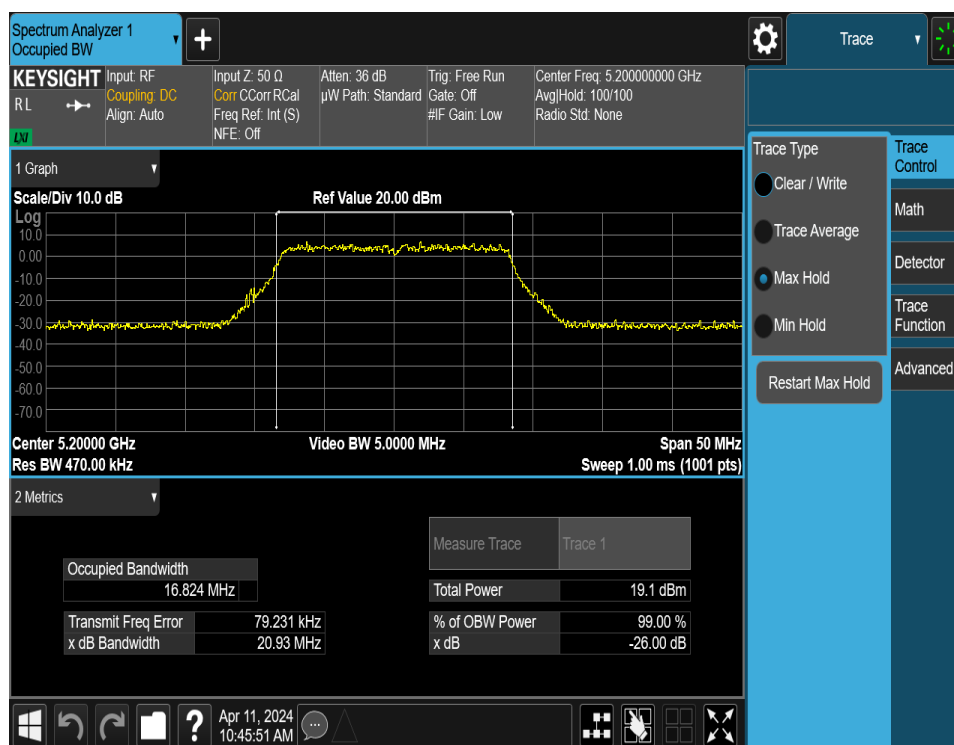
Plot 7-26. 26dB Bandwidth Plot MIMO ANT2 (802.11a (UNII Band 1) – Ch. 40)
