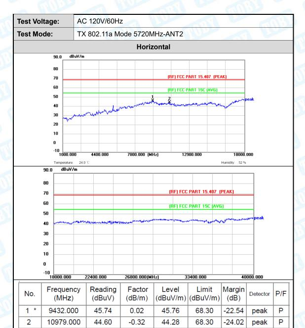
1. Corr. = Antenna Factor (dB/m) + Cable Loss (dB)
