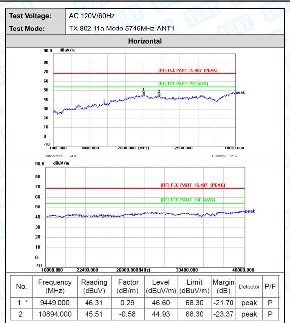
1. Corr. = Antenna Factor (dB/m) + Cable Loss (dB)
