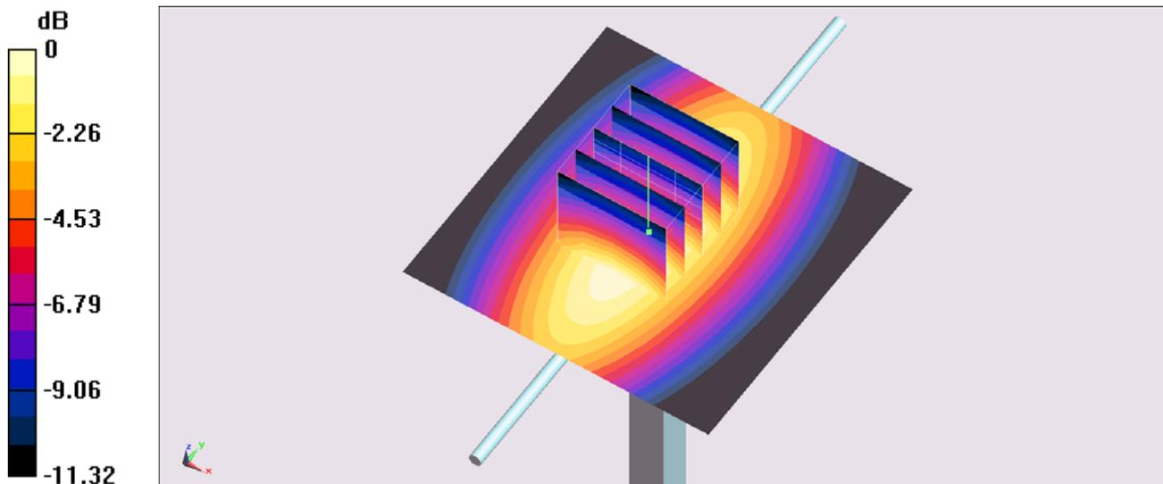
0 dB =  $2.87 \text{ W/kg} = 4.58 \text{ dBW/kg}$
