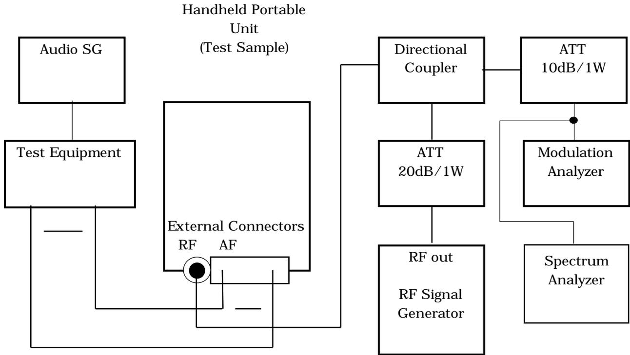
TRANSMITTER TEST SET-UP (2)
