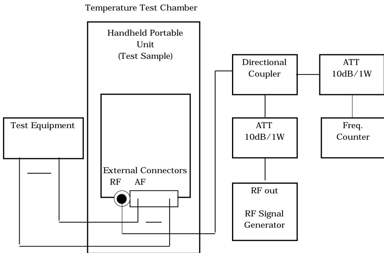
TRANSMITTER TEST SET-UP (3)
