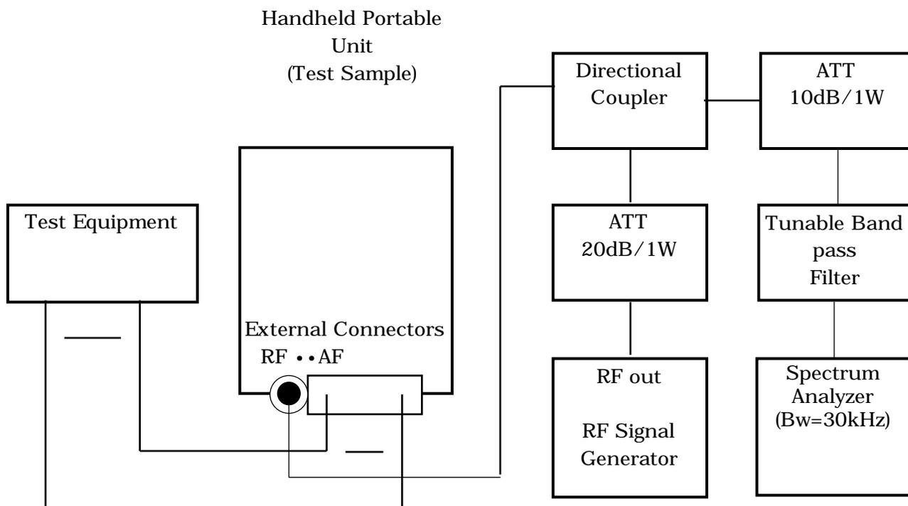
TRANSMITTER TEST SET-UP (4)
