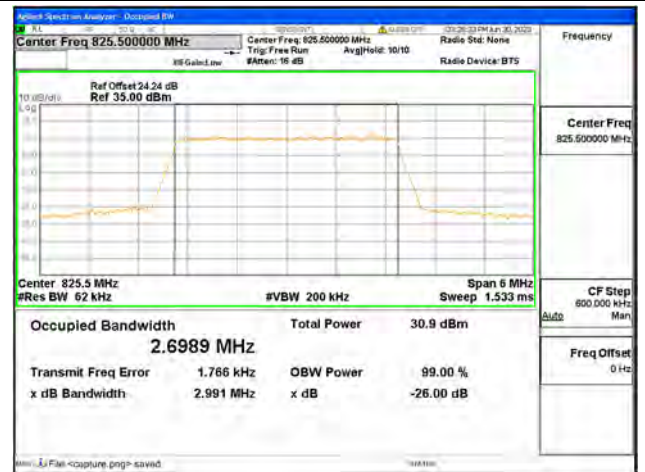
Band26 Part22 / 3MHz / QPSK/ Low CH
