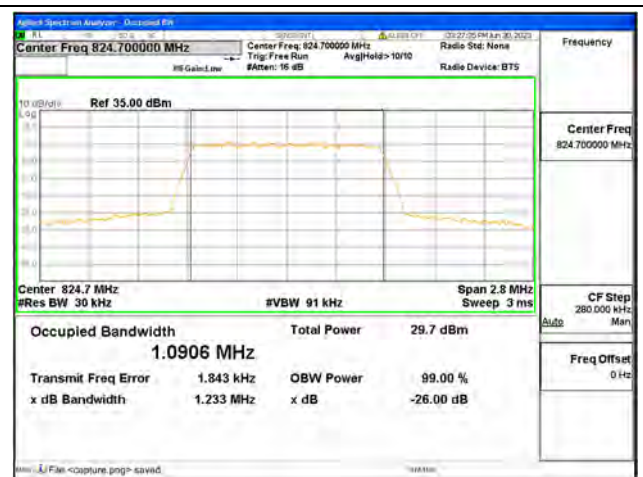
Band26 Part22 / 1.4MHz / 16QAM/ Low CH
