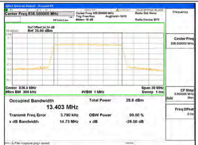
Band26 Part22 / 15MHz / 64QAM/ Mid CH
