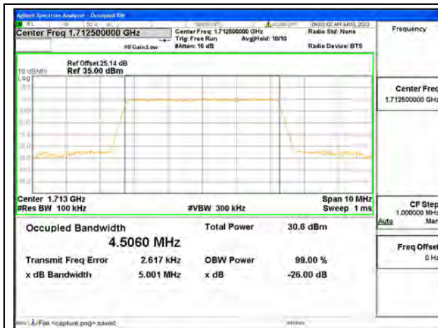
Band66 / 5MHz / QPSK/ Low CH
