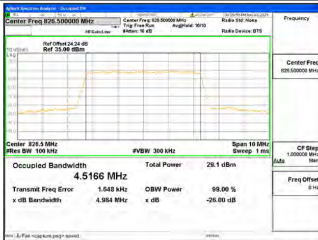
Band26 Part22 / 5MHz / 64QAM/ Low CH
