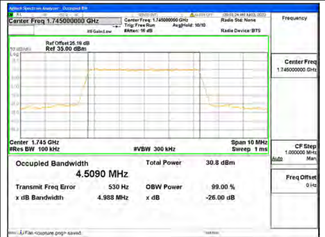
Band66 / 5MHz / QPSK/ Mid CH
