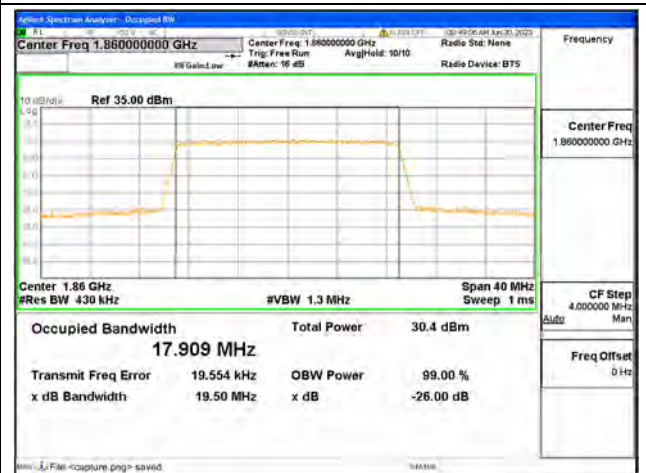
Band25 / 20MHz / 64QAM/ Low CH
