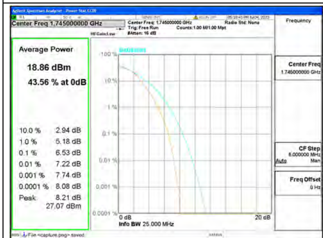
Band4 / 20MHz / High CH / 16QAM
