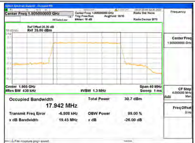
Band25 / 20MHz / 64QAM/ High CH
