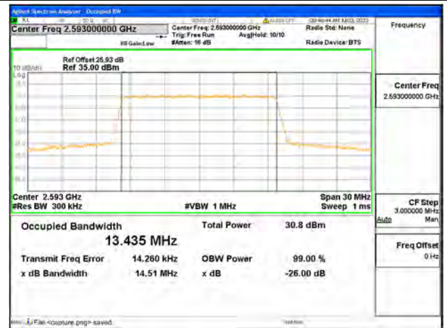
Band41 / 15MHz / QPSK/ Mid CH
