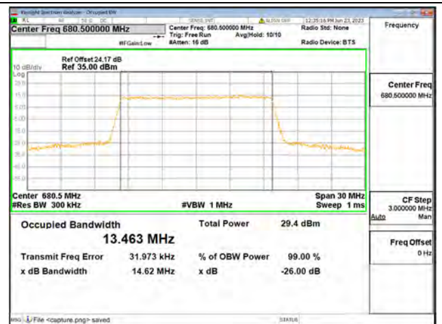
Band71 / 15MHz / 64QAM/ Mid CH
