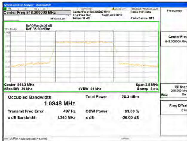
Band26 Part22 / 1.4MHz / 64QAM/ High CH
