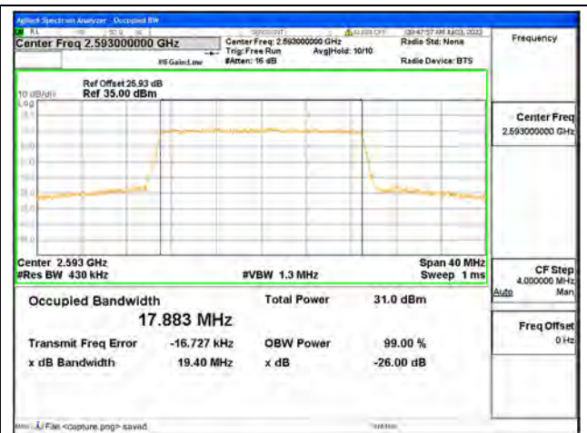
Band41 / 20MHz / 16QAM/ Mid CH
