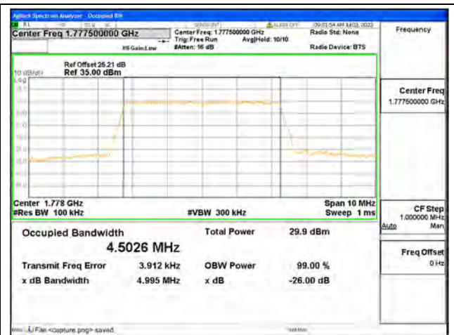
Band66 / 5MHz / 16QAM/ High CH
