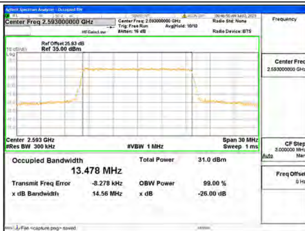
Band41 / 15MHz / 16QAM/ Mid CH
