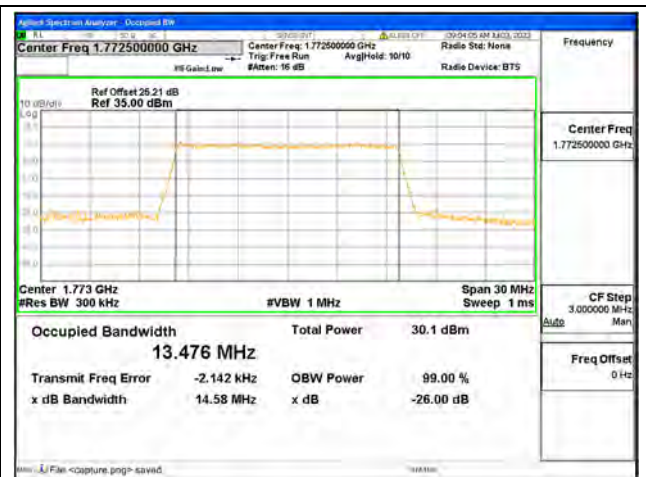
Band66 / 15MHz / 16QAM/ High CH
