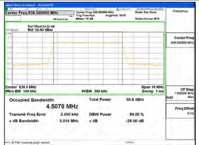
Band26 Part22 / 5MHz / QPSK/ Mid CH
