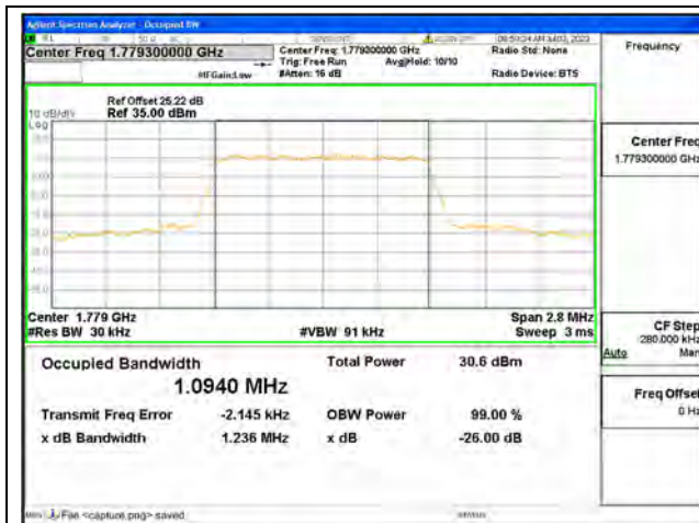
Band66 / 1.4MHz / QPSK/ High CH
