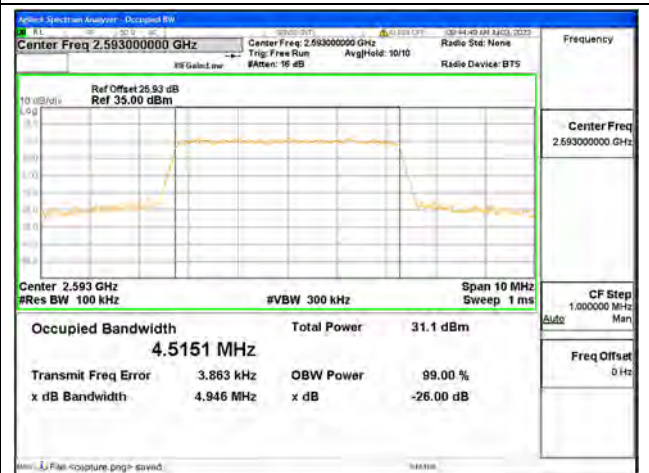
Band41 / 5MHz / 64QAM/ Mid CH
