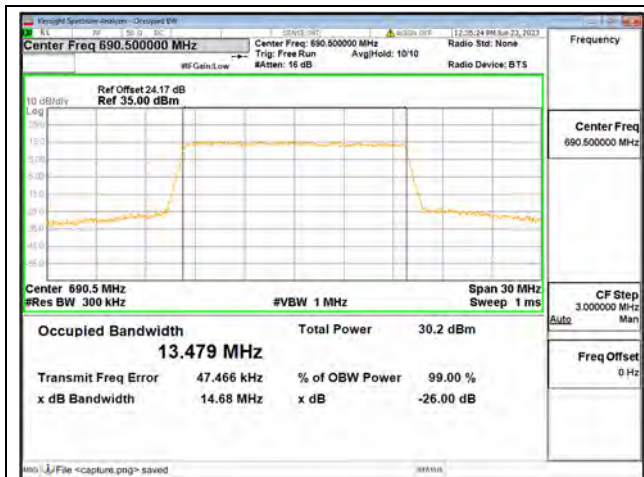
Band71 / 15MHz / QPSK/ High CH
