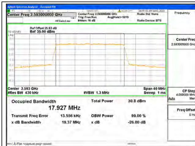
Band41 / 20MHz / QPSK/ Mid CH
