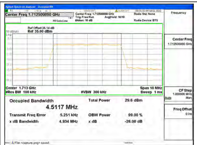
Band66 / 5MHz / 16QAM/ Low CH
