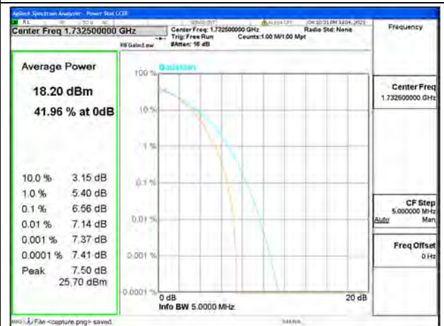
Band4 / 1.4MHz / Mid CH / 64QAM
