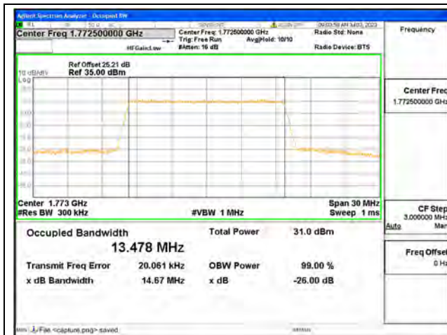
Band66 / 15MHz / QPSK/ High CH
