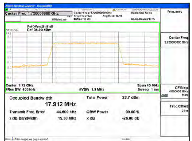
Band66 / 20MHz / 64QAM/ Low CH
