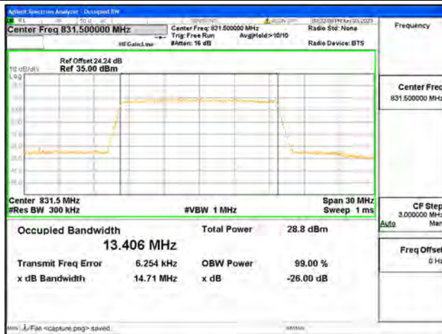
Band26 Part22 / 15MHz / 64QAM/ Low CH
