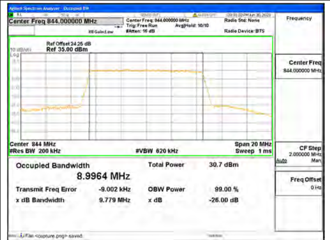
Band26 Part22 / 10MHz / QPSK/ High CH
