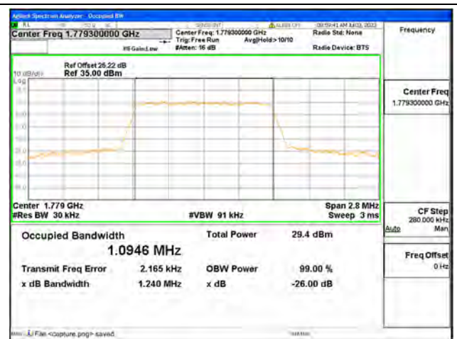
Band66 / 1.4MHz / 16QAM/ High CH
