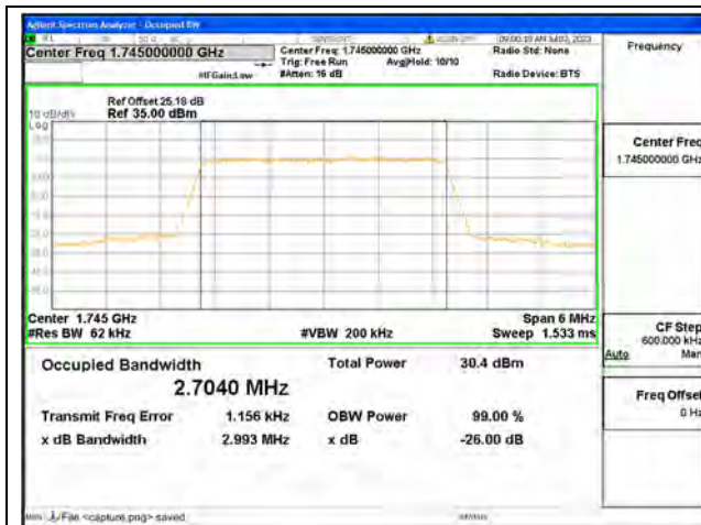
Band66 / 3MHz / QPSK/ Mid CH
