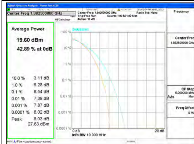
Band25 / 10MHz / Mid CH / 64QAM
