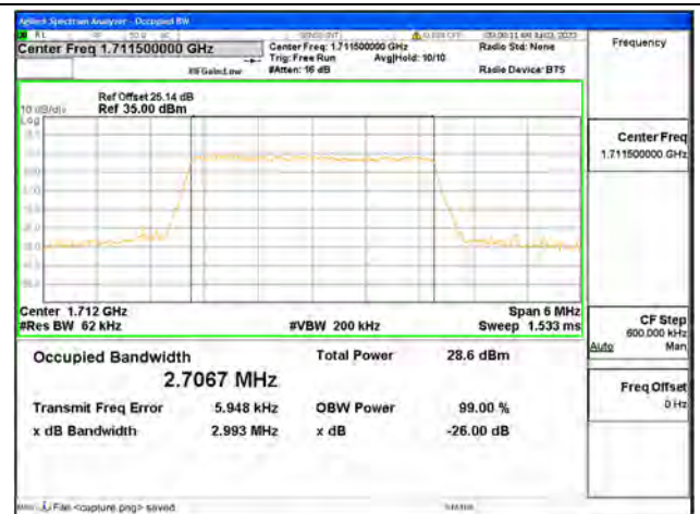
Band66 / 3MHz / 64QAM/ Low CH
