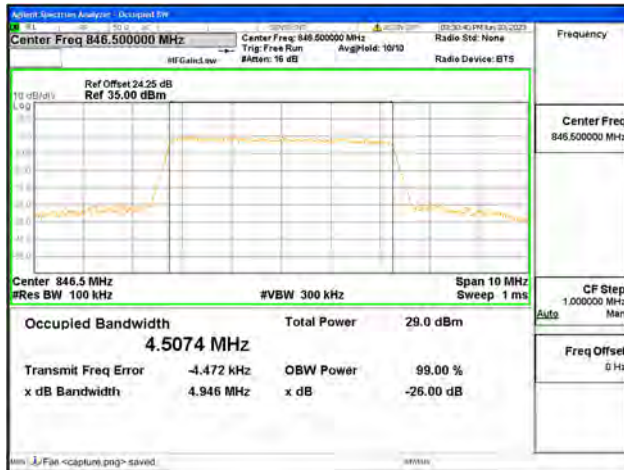
Band26 Part22 / 5MHz / 64QAM/ High CH
