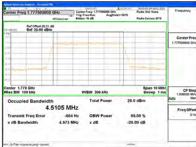
Band66 / 5MHz / 64QAM/ High CH
