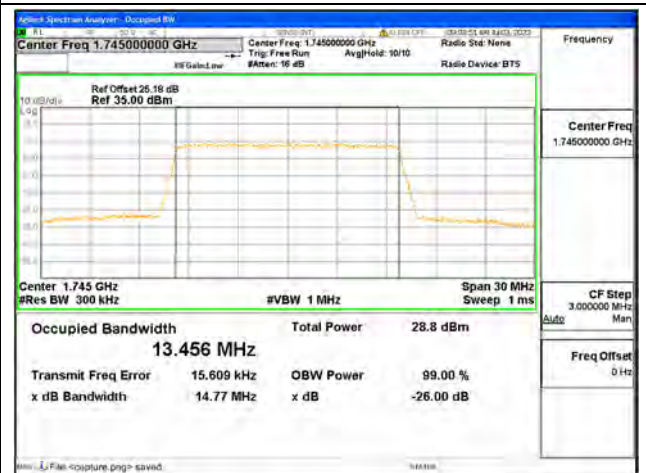
Band66 / 15MHz / 64QAM/ Mid CH
