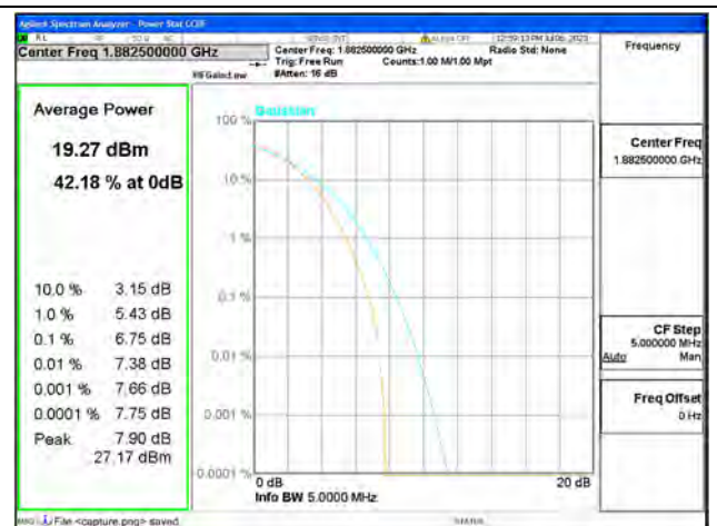
Band25 / 1.4MHz / Mid CH / 64QAM
