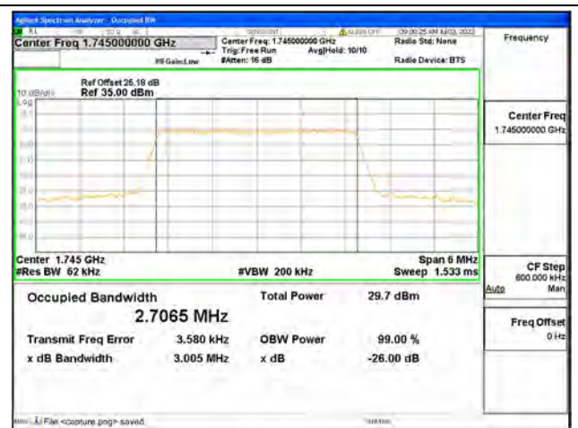
Band66 / 3MHz / 16QAM/ Mid CH
