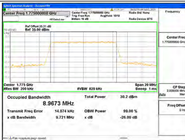
Band66 / 10MHz / 16QAM/ High CH
