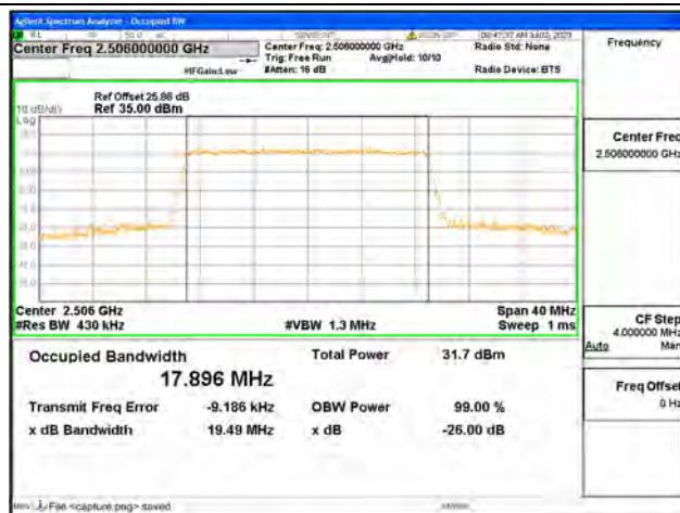
Band41 / 20MHz / 16QAM/ Low CH
