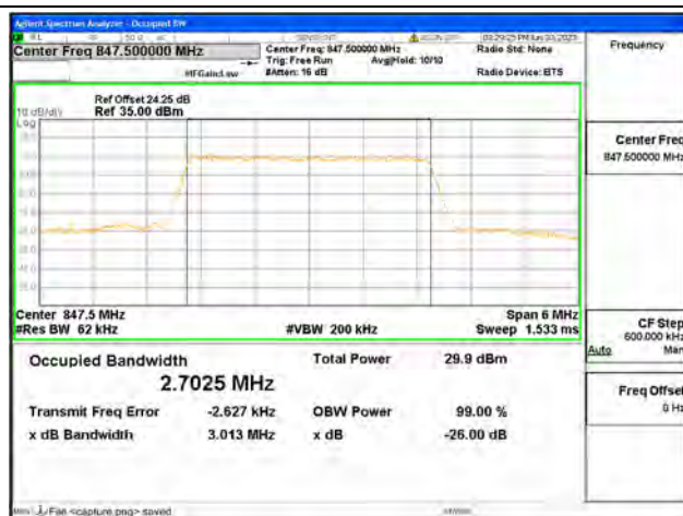
Band26 Part22 / 3MHz / 16QAM/ High CH
