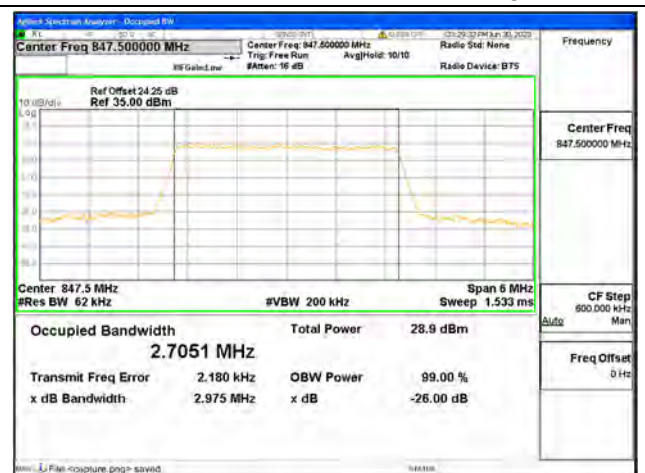
Band26 Part22 / 3MHz / 64QAM/ High CH
