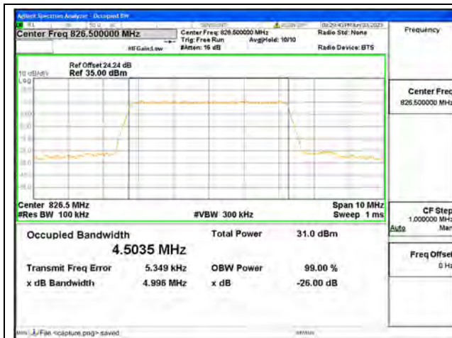
Band26 Part22 / 5MHz / QPSK/ Low CH
