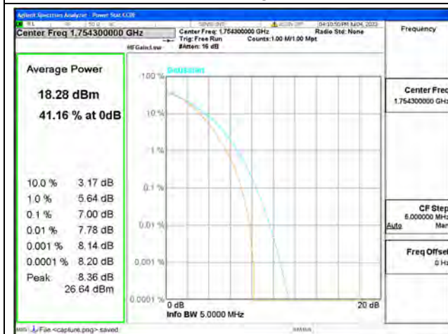
Band4 / 1.4MHz / High CH / 64QAM
