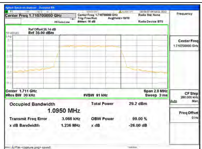
Band66 / 1.4MHz / 16QAM/ Low CH
