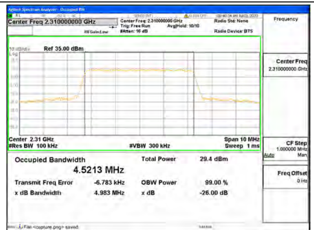
Band30 / 5MHz / 64QAM/ Mid CH
