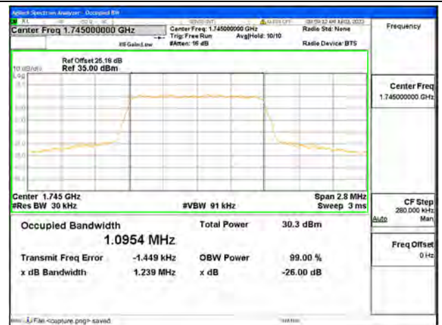
Band66 / 1.4MHz / QPSK/ Mid CH
