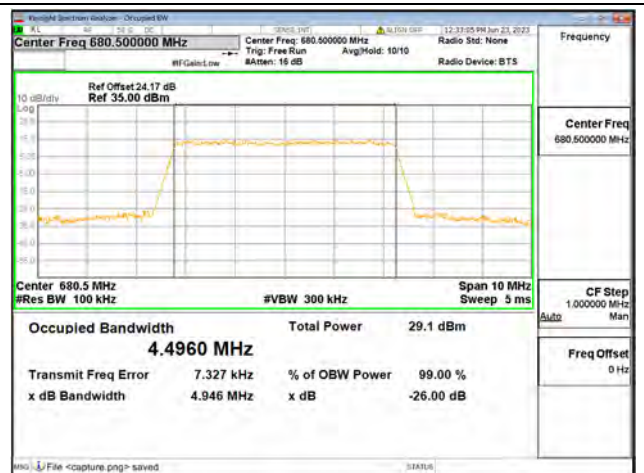
Band71 / 5MHz / 64QAM/ Mid CH
