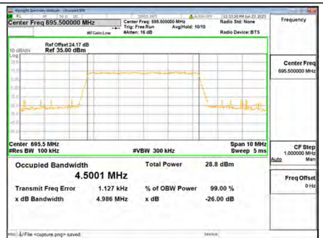
Band71 / 5MHz / 16QAM/ High CH
