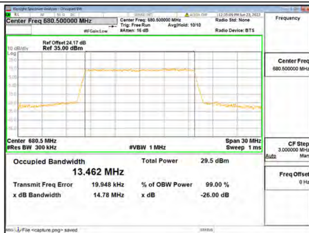
Band71 / 15MHz / 16QAM/ Mid CH
