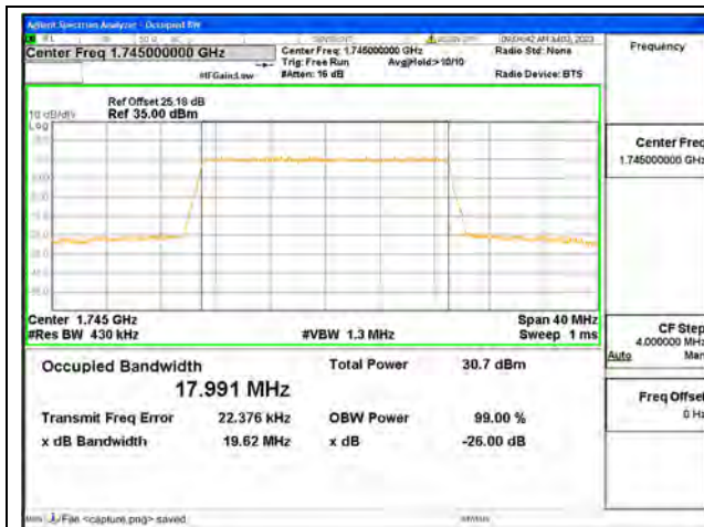
Band66 / 20MHz / QPSK/ Mid CH
