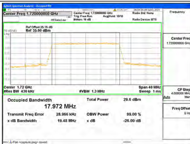
Band66 / 20MHz / 16QAM/ Low CH
