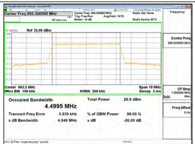
Band71 / 5MHz / 16QAM/ Low CH
