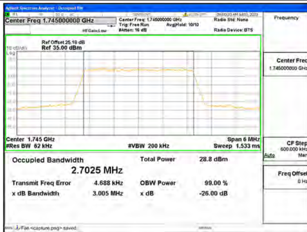
Band66 / 3MHz / 64QAM/ Mid CH
