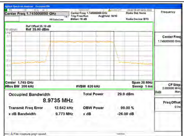
Band66 / 10MHz / 16QAM/ Mid CH
