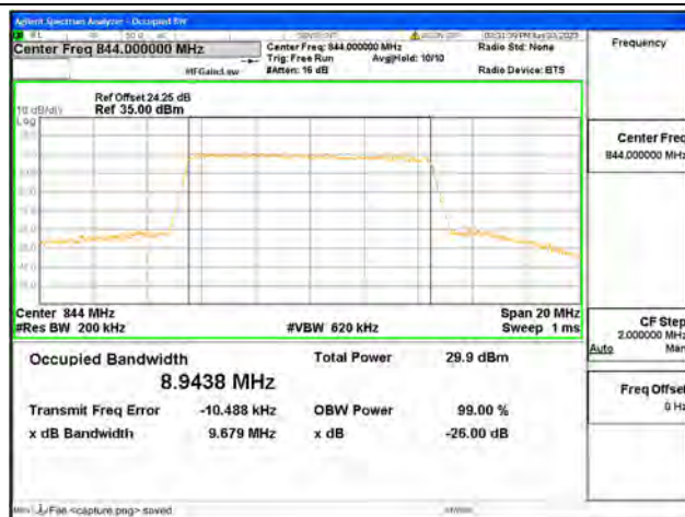
Band26 Part22 / 10MHz / 16QAM/ High CH
