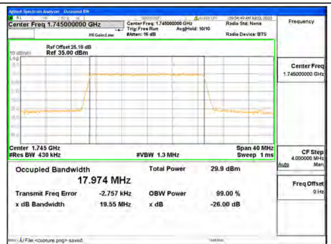
Band66 / 20MHz / 16QAM/ Mid CH
