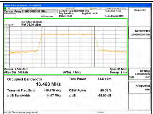
Band41 / 15MHz / 16QAM/ Low CH
