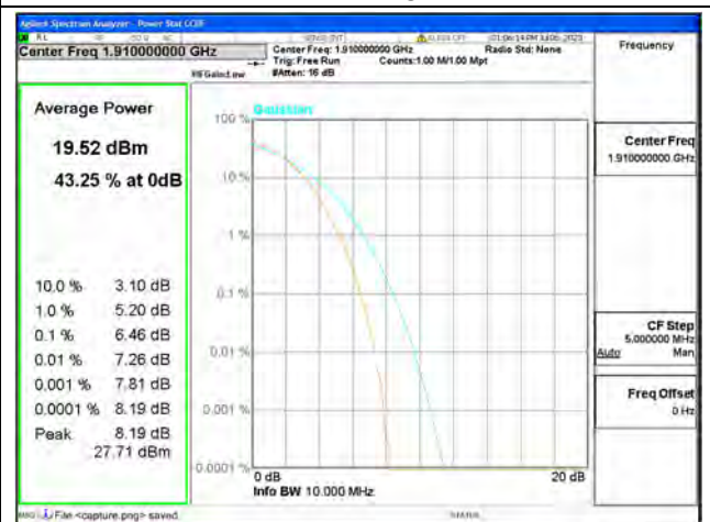
Band25 / 10MHz / High CH / 64QAM
