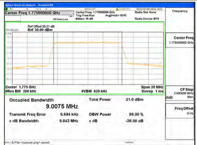
Band66 / 10MHz / QPSK/ High CH
