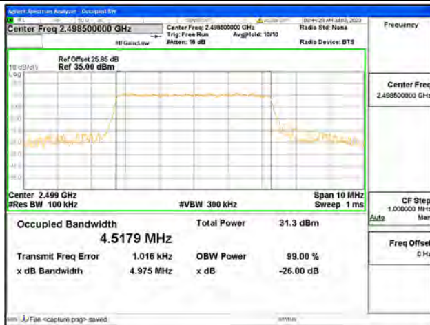
Band41 / 5MHz / 64QAM/ Low CH
