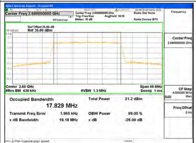
Band41 / 20MHz / 64QAM/ High CH
