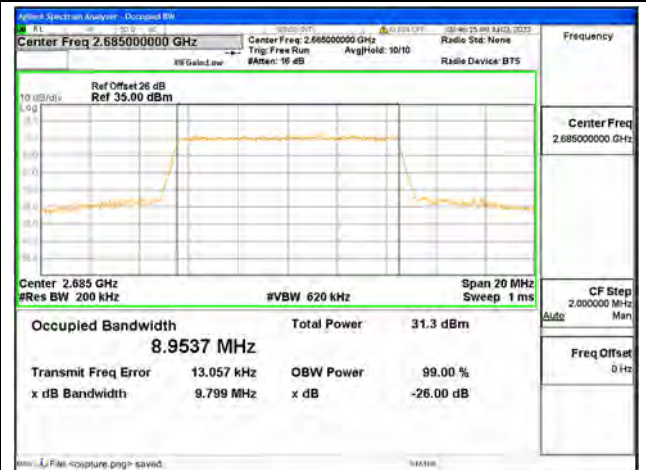
Band41 / 10MHz / 64QAM/ High CH
