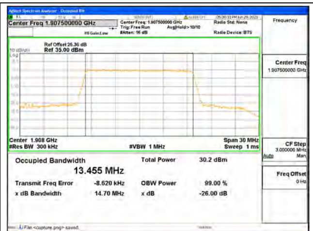
Band25 / 15MHz / 16QAM/ High CH
