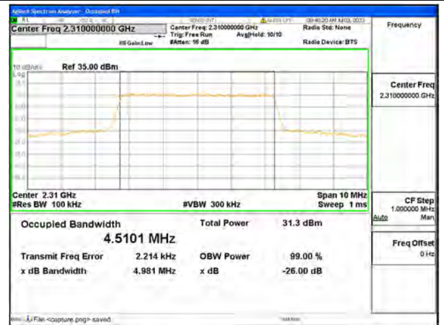
Band30 / 5MHz / QPSK/ Mid CH
