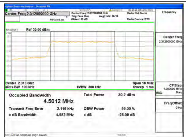
Band30 / 5MHz / 16QAM/ High CH
