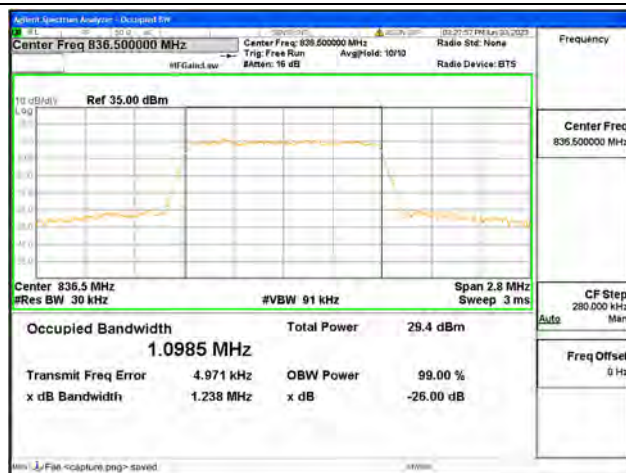
Band26 Part22 / 1.4MHz / 16QAM/ Mid CH
