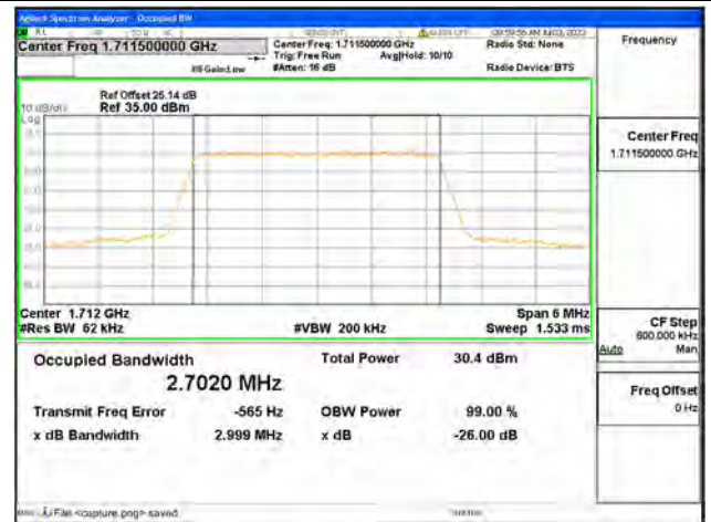
Band66 / 3MHz / QPSK/ Low CH
