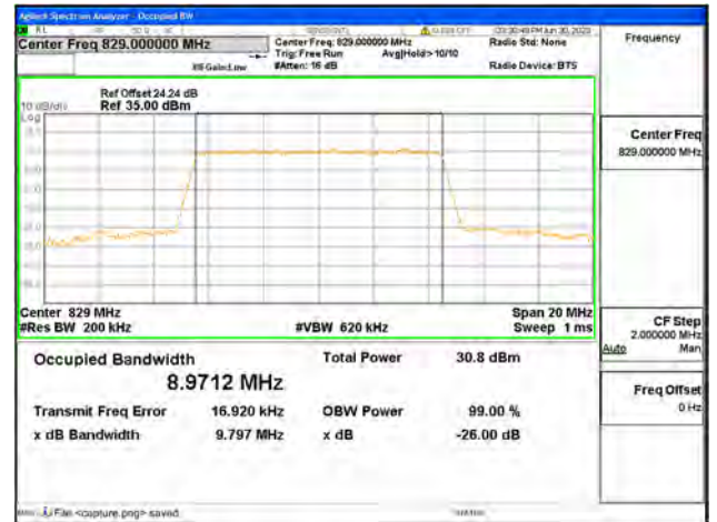
Band26 Part22 / 10MHz / QPSK/ Low CH
