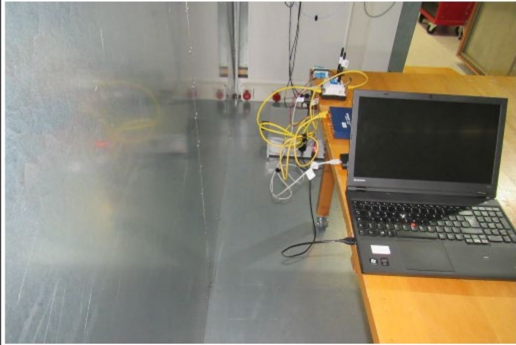
Test setup AC-Powerline CE
