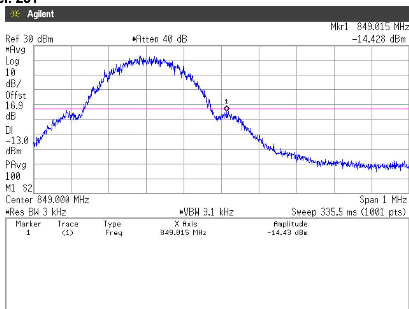
**(Spurious Emissions)****Note: Conducted spurious test was measured in the worst case of conducted output power.****Channel: 128**
