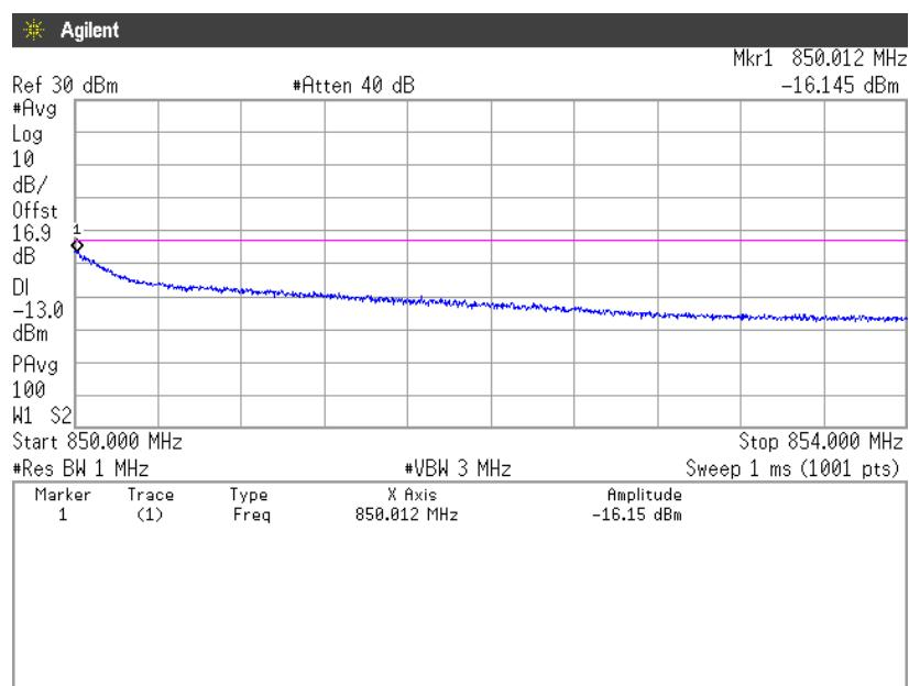
**(Spurious Emissions)****Note: Conducted spurious test was measured in the worst case of conducted output power.****Channel: 4132**
