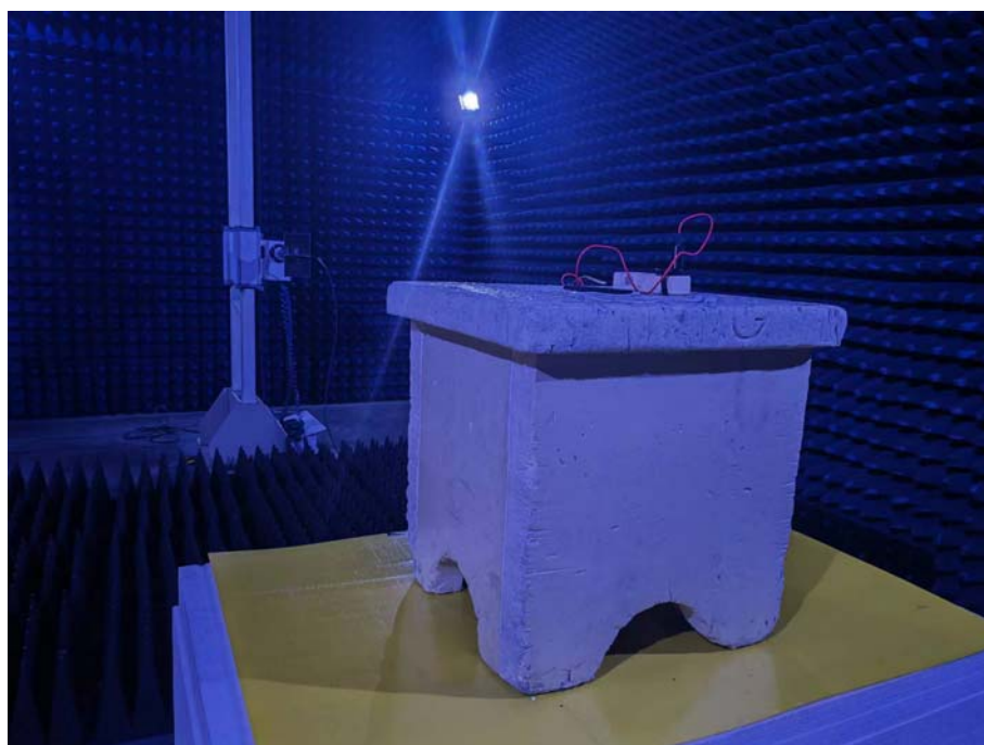
Photo of Radiated Emission Measurement (Above 1GHz)
