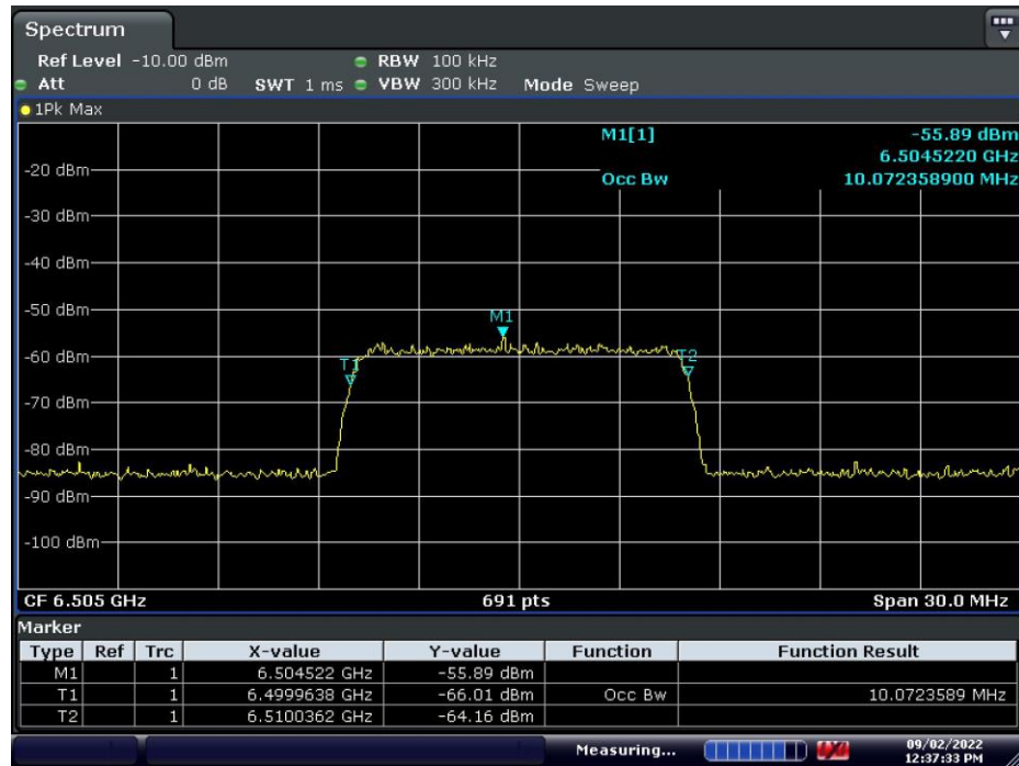
Plot 7-567. AWGN Signal – UNII 6 – 160MHz – Mid
