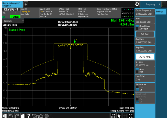
Plot 7-560. In-Band Emission Plot SDM Antenna 4a (160MHz 802.11ax (UNII Band 8) – Ch. 207, MCS11)
