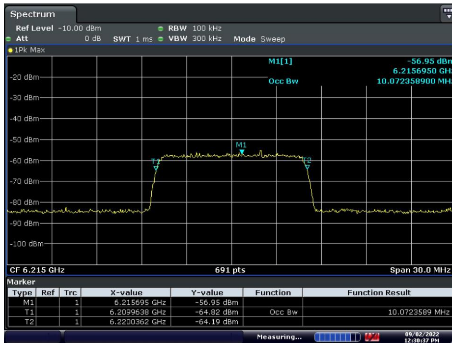
Plot 7-561. AWGN Signal – UNII 5 – 20MHz
