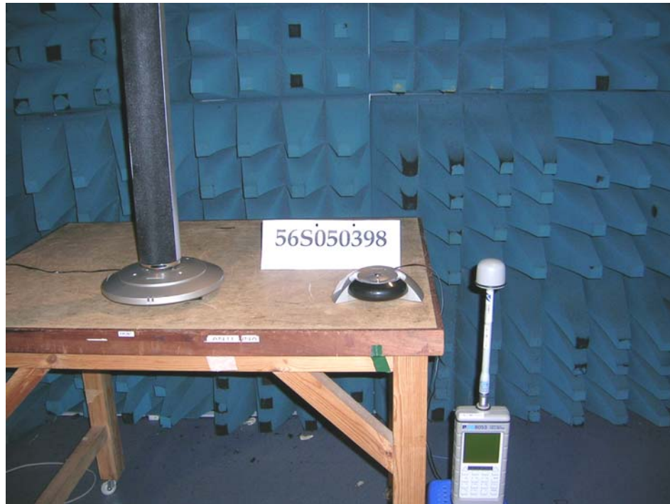
Maximum Permissible Exposure Measurement Test Setup (Wireless Transmitter)
