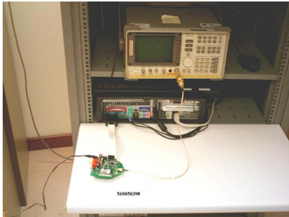
Carrier Frequency Separation Measurement Test Setup
