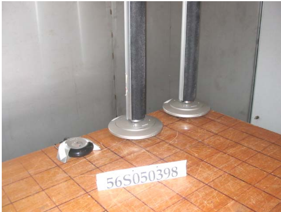
Conducted Emissions Setup (Front View)
