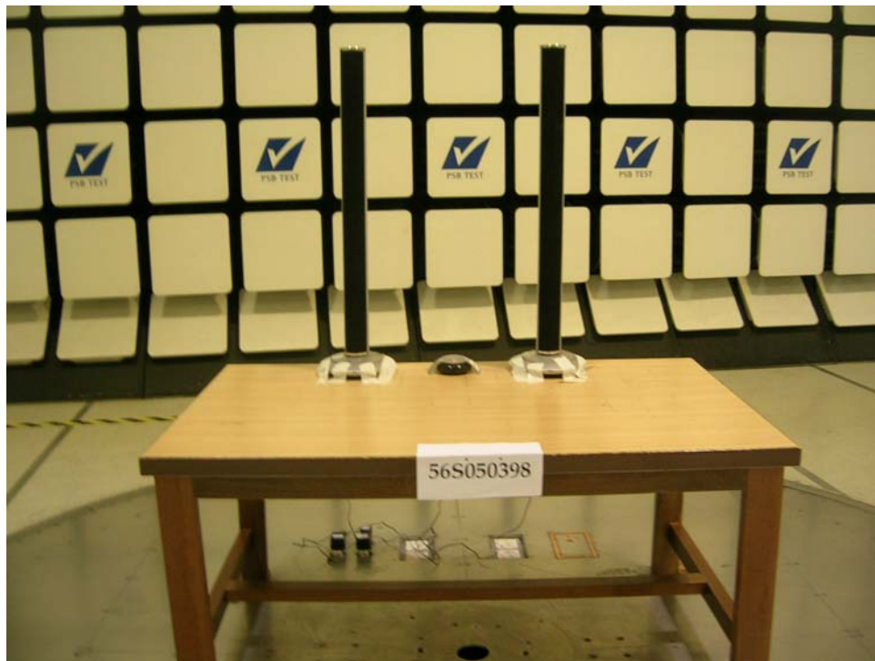
Radiated Emissions Setup (Front View)
