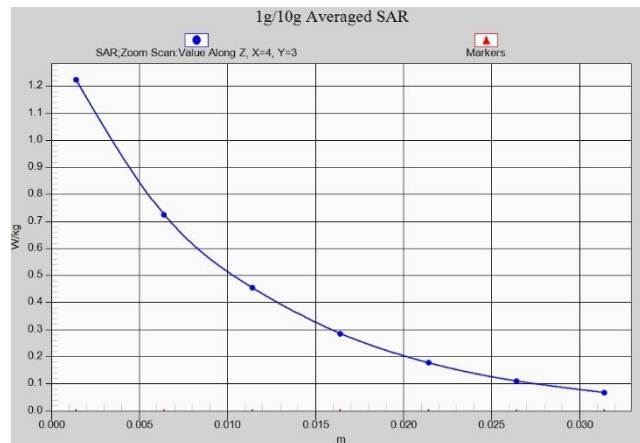
Z-Scan at power reference point (LTEB66)
