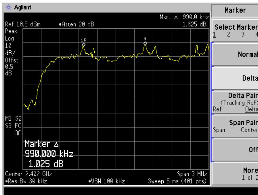
Channel Spacing (Middle CH=1MHz)
