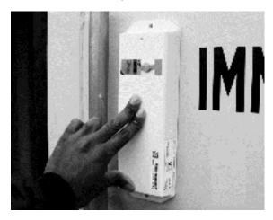
6. Insert your fastener of choice into the holes and use the appropriate tools to secure the module to the asset.
