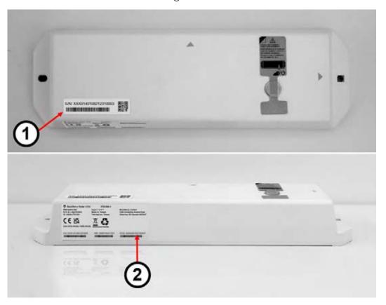
2. Once you have installed the module on the asset, create a record of the module-toasset-to-accessory pairing within the BlackBerry Radar Mobile App by recording the asset identifier and scanning the module identifier for the BlackBerry Radar H2M IS device and associated accessories.
