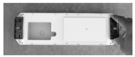
6. Ensure the arrow on the top of the housing is pointing to the sky. Place the assembly on the door, aligning the holes on the module with the holes you drilled into the door.
