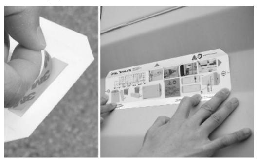
3. Using a drill bit, drill a hole through each of the cross hairs on the template. This will create two holes you will use to mount the module.
