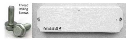
Thread rolling screws create their own threads within the thickness of the asset's installation surface. These threads allow the device to be secured to the asset, without the use of a secondary fastener, like a lock nut (although some thread rolling screws can be used with some lock nuts, for extra holding opportunity).
