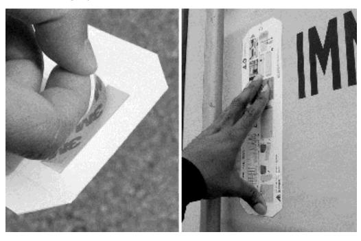
It is recommended that you install the module as level as possible on the asset. Angled installations are not supported. To help ensure the module is level, you may try one of the following techniques.
