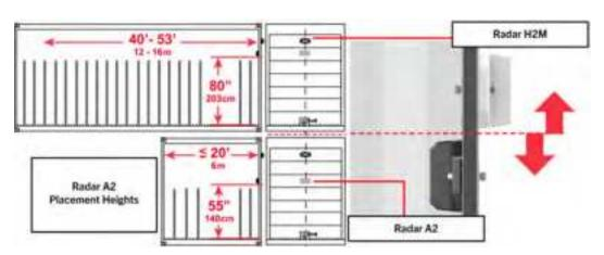
Horizontal and Vertical installation orientations are supported. When determining the preferred installation location and orientation for your module, be sure to install the module in a location that does not cover any important container markings. If your container's markings, and door geometry require placement of the Radar H2M within angled door geometry, you will require the use of the Radar H2M Container Accessory.
