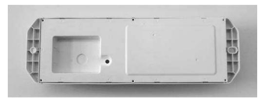
4. Using a Torx T6 screwdriver, install the screws to secure the battery door. **IMPORTANT:** Screw torque must be 2.6 in-lb (0.3 N-m).
