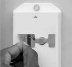
B. Continue to lift the magnet tape and fully remove the magnet tape from the module. Lifting the magnet tape will remove the magnet from the magnet ring.
