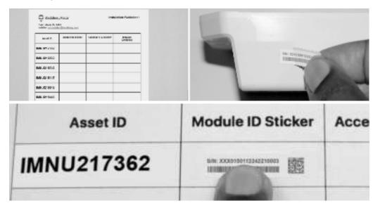
**Tip:** For modules that have previously been transferred to new assets, the temporary S/N label may no longer be in place. If this is the case, you will need to write the module identifier (S/N) for each module on the installation worksheet.
