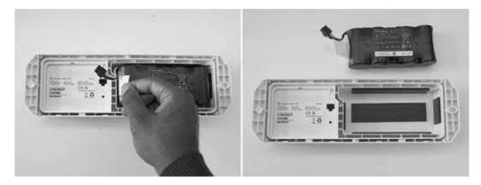
4. Remove the battery from the battery compartment by grasping the pull tab and lifting the battery out of the compartment.
