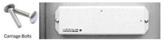
Carriage bolts are like standard bolts, but with a different head. The head of a carriage bolt is a domed shape with a square shank protruding from its flat side. The square shank on the base is inserted into the square slots on the module. The square slot holds the bolt in place when a nut is fastened onto it--while a standard bolt would require a tool to hold the bolt for fastening the nut.
