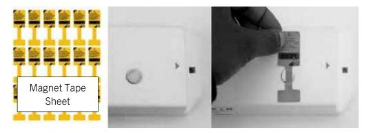
**IMPORTANT:** When the battery is connected, never ship the module without the magnet in place. The magnet is necessary to keep the module powered off during transit.
