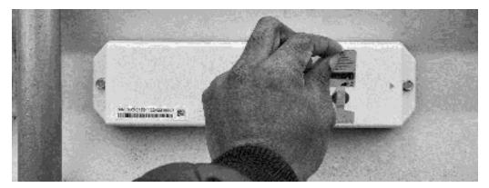
B. Lift the corner of the magnet tape and fully remove the magnet tape from the module. Lifting the magnet tape will remove the magnet from the magnet ring.
