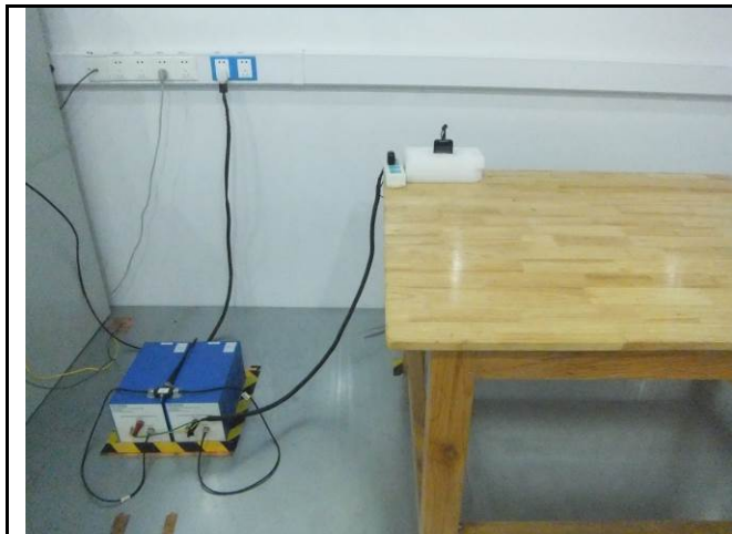
Conducted Emissions Test Setup Front View
