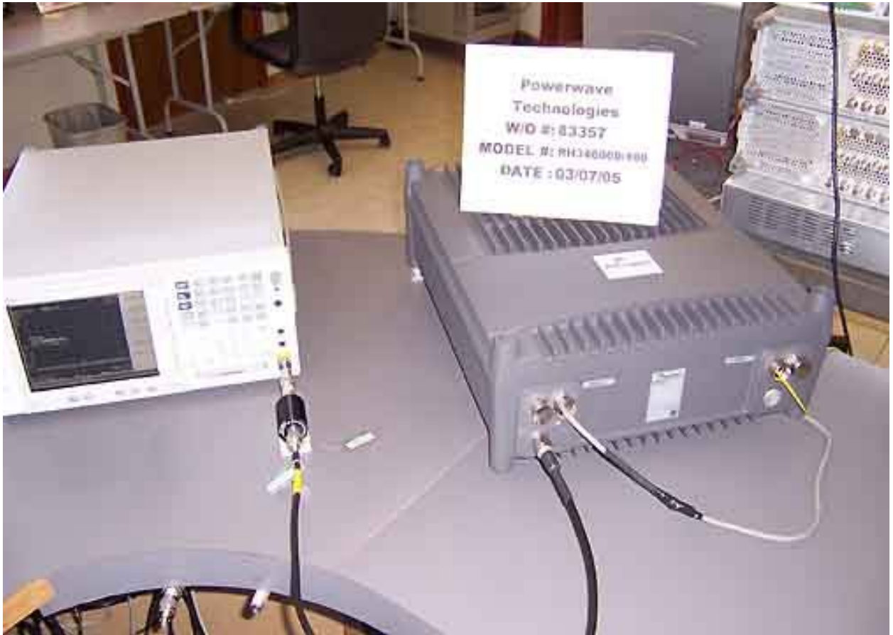
PHOTOGRAPH SHOWING DIRECT CONNECT TEST SETUP
