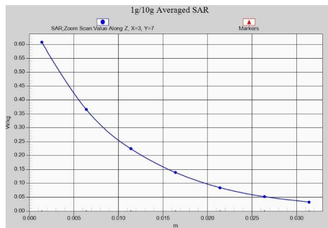
Fig. 1-8 Z-Scan at power reference point (WCDMA1700)
