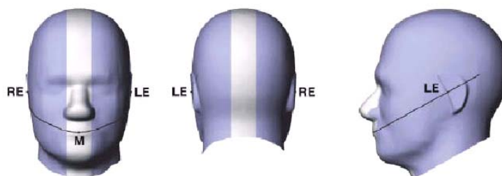
Figure 8.1 shows the front,, back and side views of the SAM Twin Phantom. The point “M” is the reference point for the center of the mouth, “LE” is the left ear reference point(ERP), and “RE” is the right ERP. The ERPs are 15mm posterior to the entrance to the Ear canal (EEC) along the B-M line (Back-Mouth), as shown in Figure 9.2. The plane Passing through the two ear canals and M is defined as the Reference Plane. The line N-F (Neck- Front) is perpendicular to the reference plane and passing through the RE (or LE) is called the Reference Pivoting Line (see Figure 8.2). Line B-M is perpendicular to the N-F line. Both N-F and B-M lines are marked on the external phantom shell to facilitate handset positioning [5]
