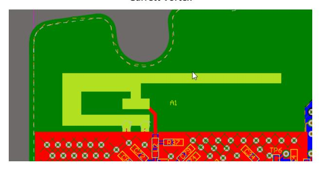
Inverted F Antenna designed in accordance with Texas Instruments Design Note SWRU120D
