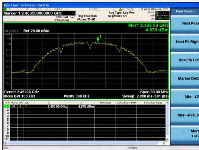
802.11b HIGH CHANNEL, CARRIER LEVEL
