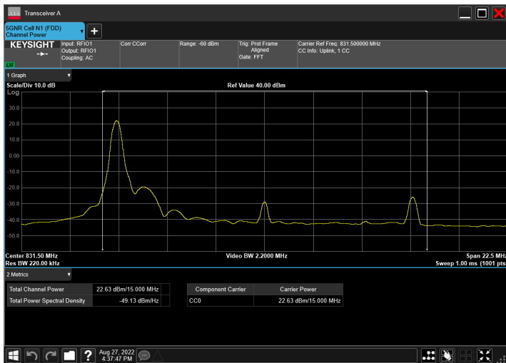
n5_15MHz_15kHz_831.5MHz_DFT-s-OFDM PI/2 BPSK_RB1@1
