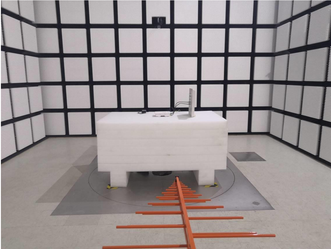
Radiated Emission Below 1GHz View - 13dBi
