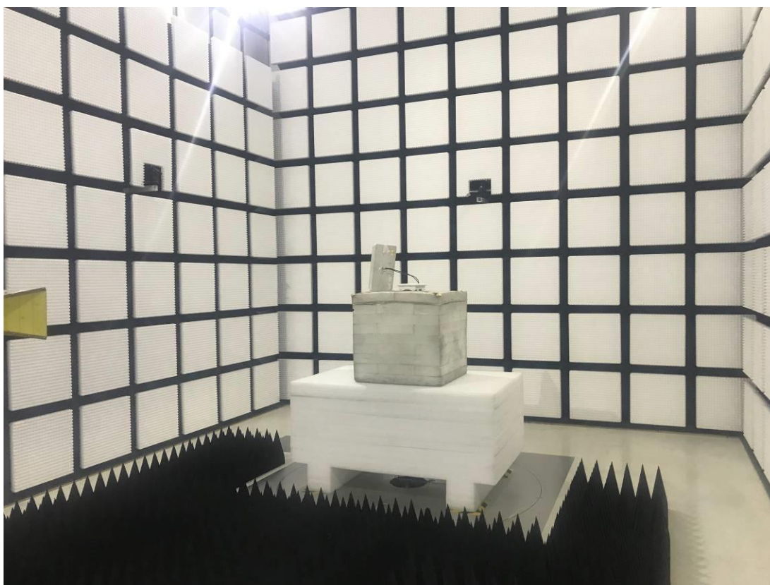
Radiated Emission Above 1GHz View -23dBi
