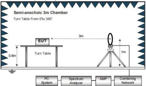
(B) Radiated Emission Test-Up Frequency 30MHz~1GHz
