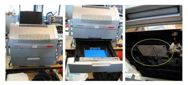
Next we show where the module is mounted on a bracket, the reader plastic enclosure snaps into the metal frame of the tray. The cabling connects on the back side.
