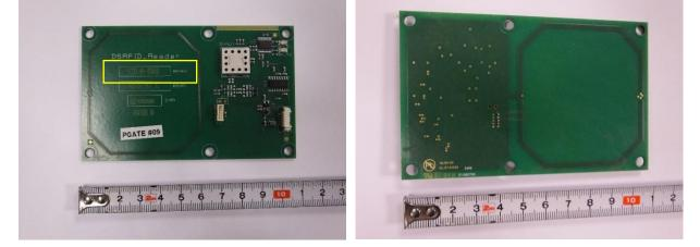
In the field BBNR2 (yellow box) the FCC ID is printed, it reads "FCC ID HPL-DSRFID-D". In the field BBNR1 the Agfa article code is printed, it reads "A800126.XX" where XX is the PCB assembly version index 07 or larger. In the field SNR1 the PCB assembly serial number is printed. The protoype used for the radio type testing is s/n RS2408059001. Note that the BBNR1, BBNR2 fields do not convey the correct descriptions, as these reflect the protoype version
