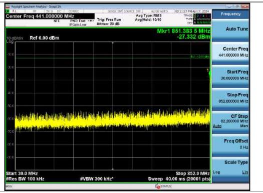
Spurious / ESMR / Downlink / LTE 5 MHz / Middle / 30 MHz ~ Low Edge - 10 MHz
