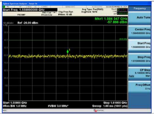
Spurious / PS Narrowband / Downlink / 12 Carrier / Additional 1559 MHz ~ 1610 MHz
