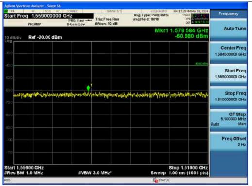
Spurious / PS Narrowband / Uplink / 12 Carrier / Additional 1559 MHz ~ 1610 MHz
