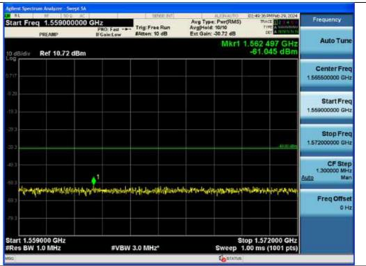
Measured Level + Ant. Gain = -61.045 dBm + 11 dBi = -50.045 dBm(E.I.R.P.) complies with the limit 27.53(f).
