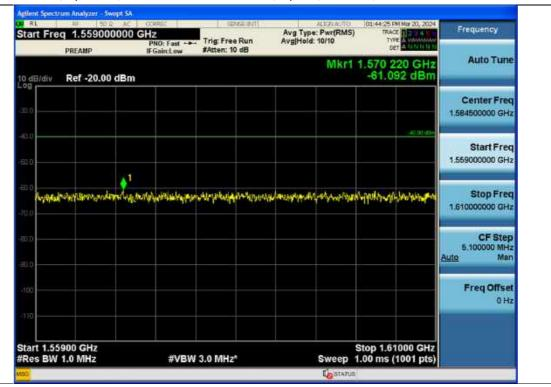
Simultaneous / Spurious / PS Narrowband + NPSPAC / Uplink / 1 Carrier / Additional 1559 MHz ~ 1610 MHz
