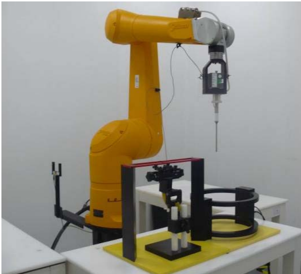
Picture 1: HAC T-Coil System Layout
