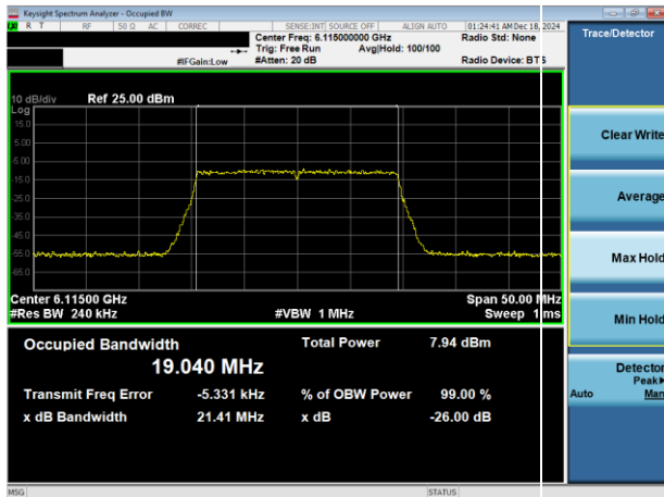
Plot 7-9. 26dB & 99% Bandwidth Plot Antenna WF7a (20MHz) 802.11ax (UNII Band 5) – Ch. 33)
