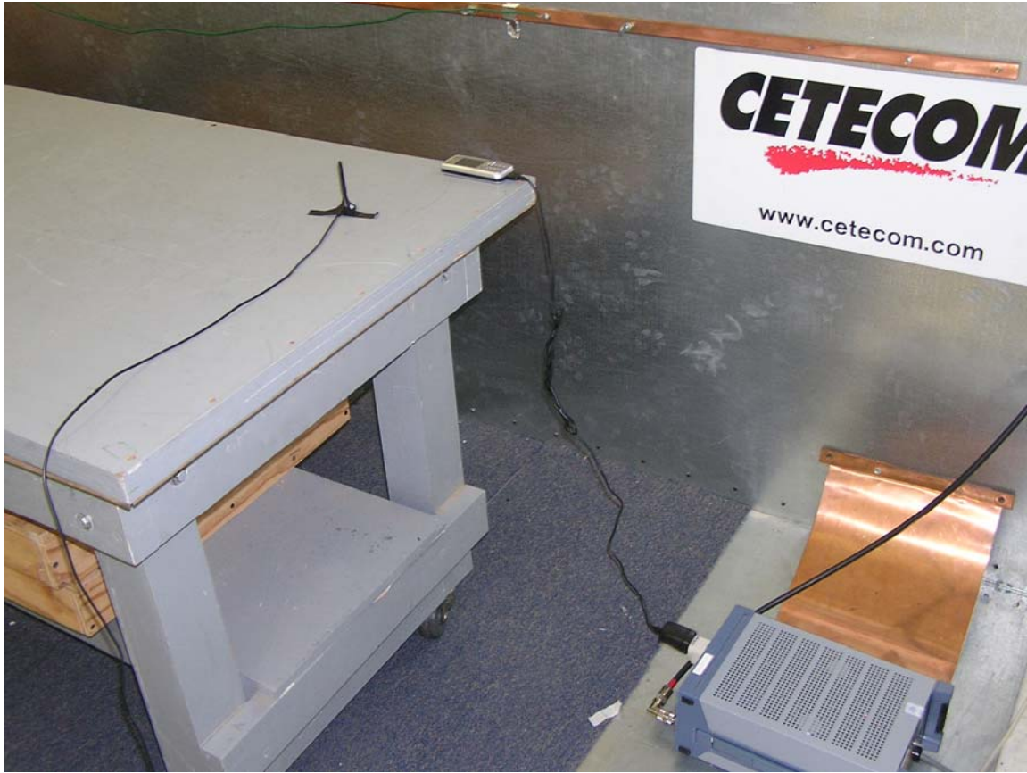
Test setup – AC Line conducted measurements
