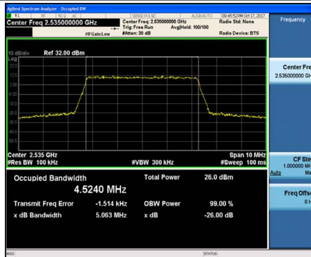
Band7_5MHz_16QAM_21100_25RB#0_4.5127_5.058_PASS
